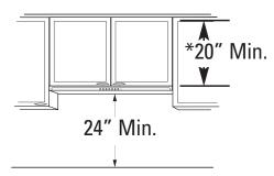
\*The cabinet must measure at least 20" from the bottom frame to the inside top. The hood housing will occupy the interior cabinet space.
